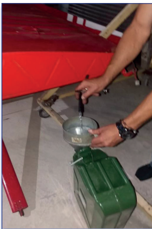
Fuel drain from the wing of a damaged aircraft
